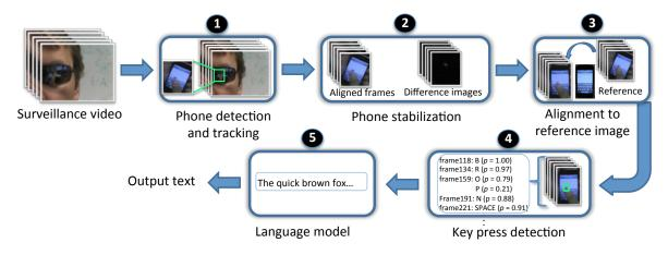
Figure 2: Overview of our approach for typed input reconstruction from video.
